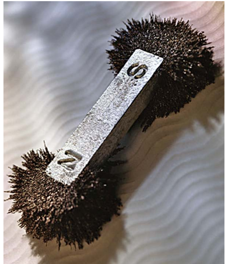
Metal filings cling to the north (N) and south (S) poles of a bar magnet.
